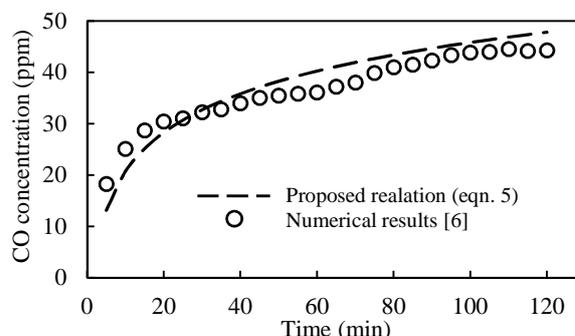
Fig. 4 Comparison of CO concentration results, normal ventilation
