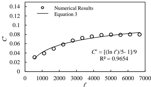
Fig. 3 Comparison of numerical results and proposed correlation
