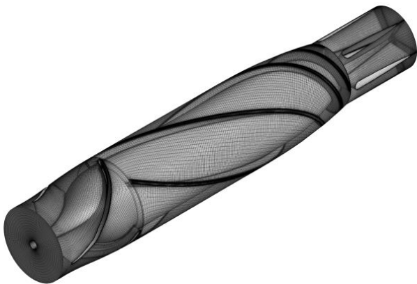
Fig. 5 Mesh used for Axial pump LVAD calculations
