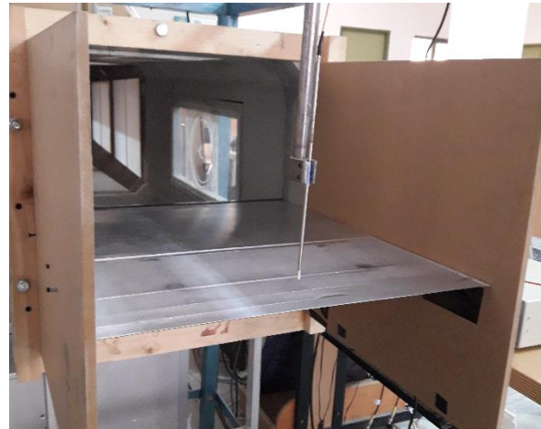
Fig. 4 Flat plate model installation in wind tunnel jet with hotwire anemometer and traverse mechanism
