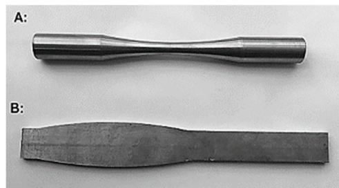
Fig. 2 A. prepared steel specimen for fatigue test. B. Copper electrode that used for machining
