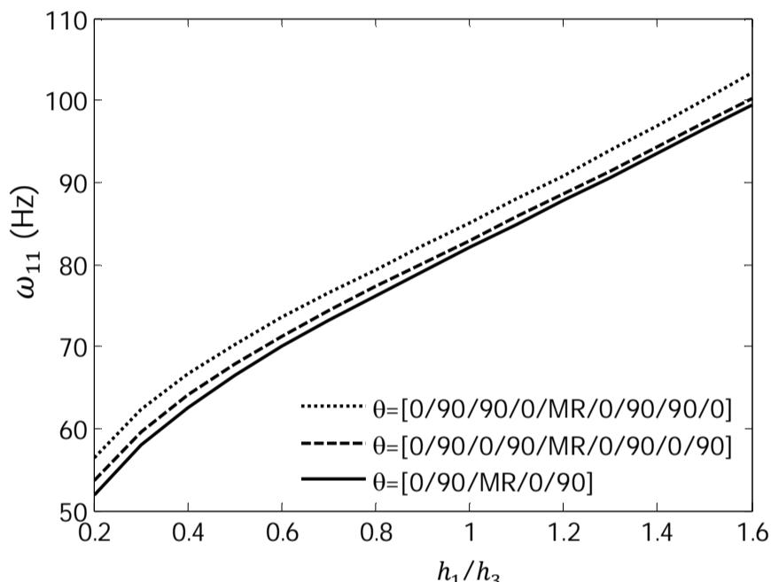
**Fig. 8** Influence of the thickness ratio ( $h_1/h_3$ ) of the constraint layer on the first mode frequency at a magnetic field of 300 Gauss
