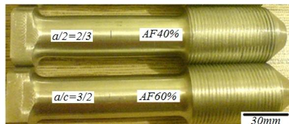
**Fig. 5** Two samples of cracked specimens with  $\xi = 0.4$
