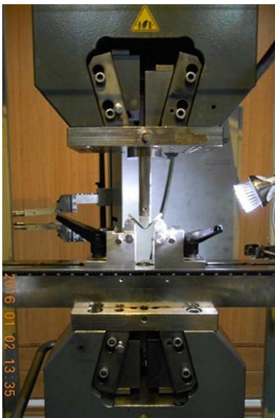
Fig. 8 The three-point bending test set-up.
