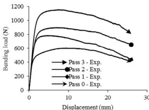
**Fig. 13** Experimental and simulation bending load-displacement curves of ECAPed Grade 2 CP-Ti specimens through 0-3 passes.
