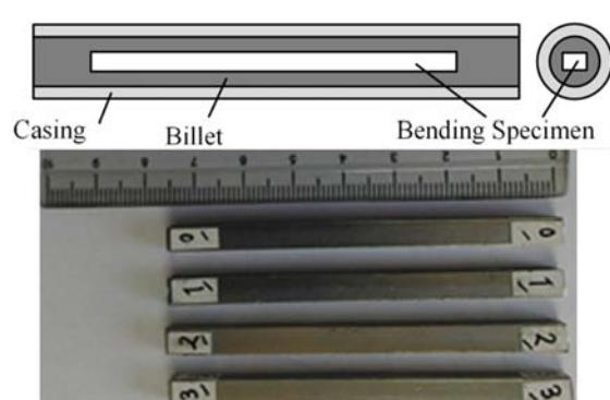
Fig. 7 Schematic and real appearance of the bending specimens before three-point bending test.
