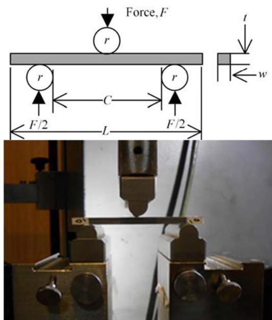
Fig. 6 Schematic and real view of fixture for the three-point bending test.
