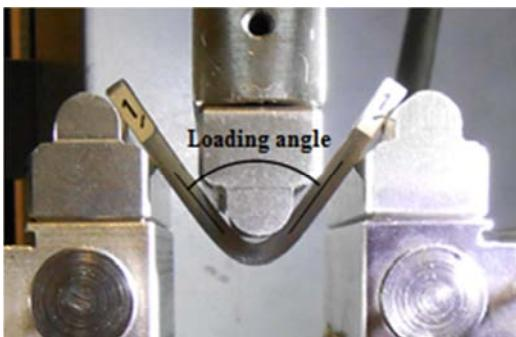
Fig. 9 Bending angle in the three point bending specimen during loading.
