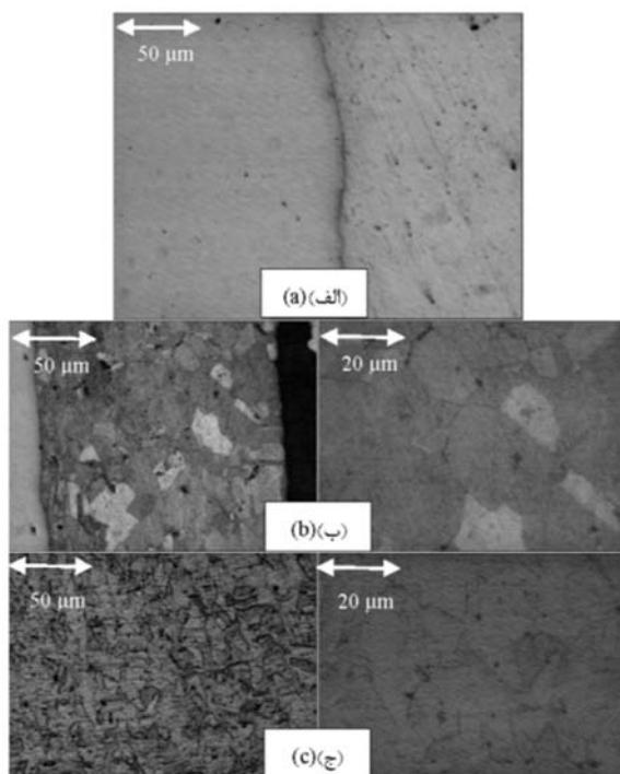
Fig. 5 Microstructure of two layered sheet in HAZ
