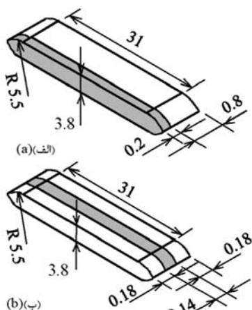
Fig. 1 Test specimens; (a) two layered sheet, (b) three layered sheet
