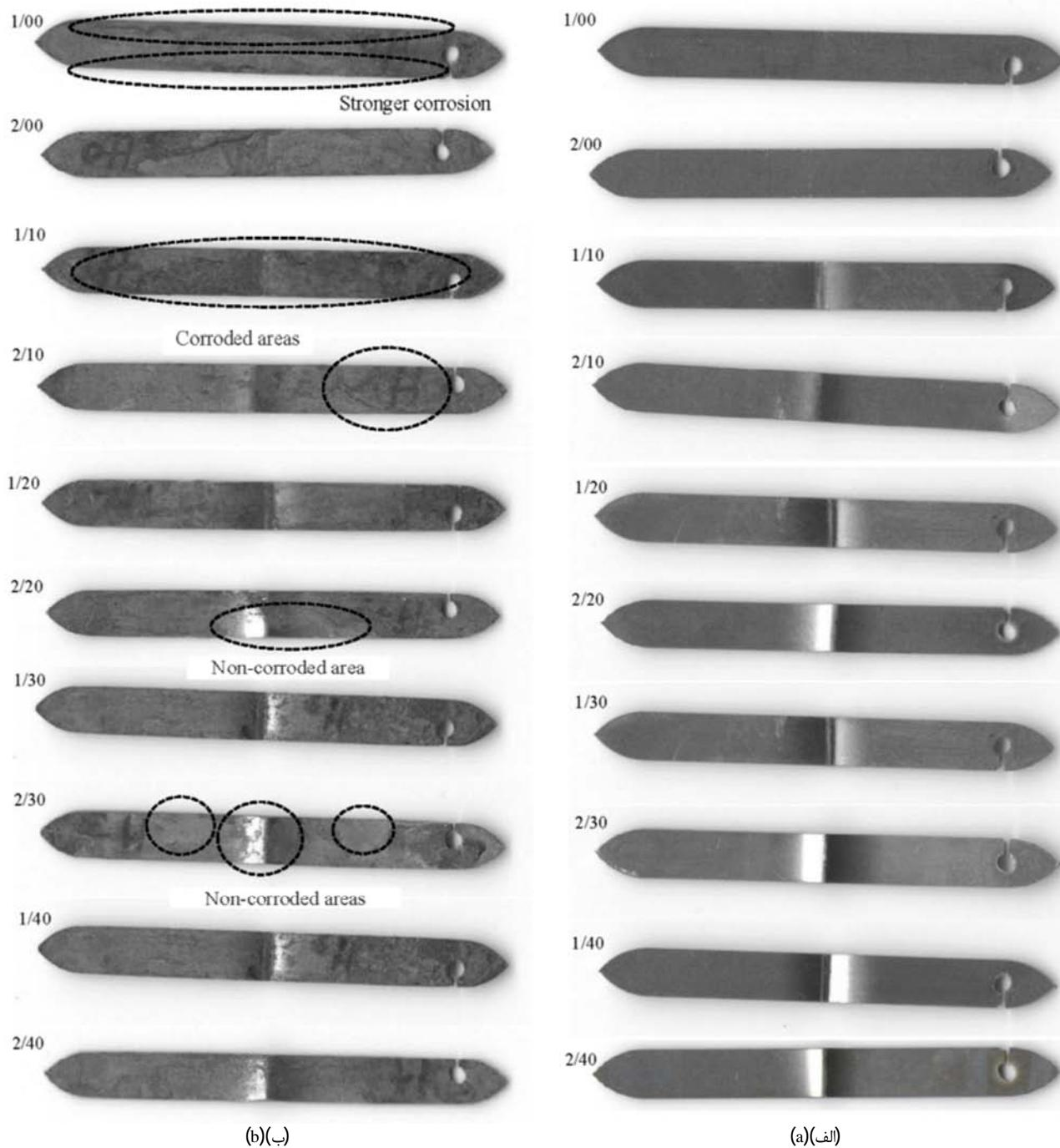
Fig. 8 Three layered sheet specimens; (a) before salt spray test, (b) after salt spray test
