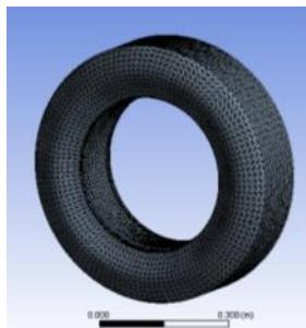
Fig. 9 Mesh of acoustic cavity model
