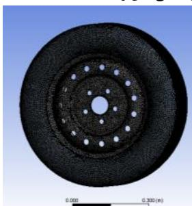
Fig. 10 The mesh generation of coupled tire, rim and fluid cavity model
