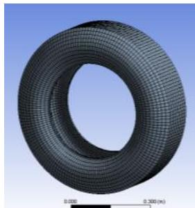
Fig. 8 Mesh of tire structural model
