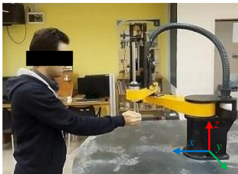
Fig. 22 Operator is forcing the FUM SCARA robot end-effector along a coordinate axis
