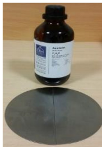
Fig. 3 Preparation of the surface of the samples by acetone
