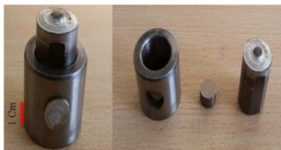
Fig. 4 Assembly and demounting of the friction welding tool
