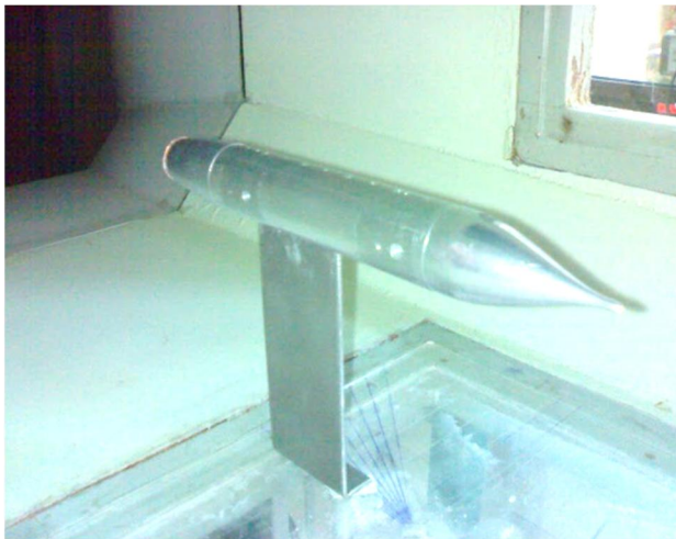
Fig. 4 model mounted on Plate type support in channel section
