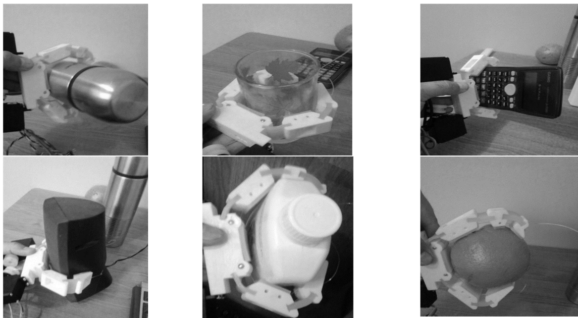
Fig. 14 The performance evaluation gripper by picking up and moving various objects
