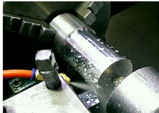
Fig. 2 Nozzle MQL, tool and workpiece setup
