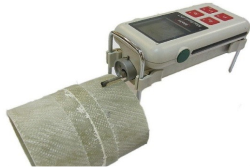
Fig. 3 Roughness measuring device and how to test surface roughness
