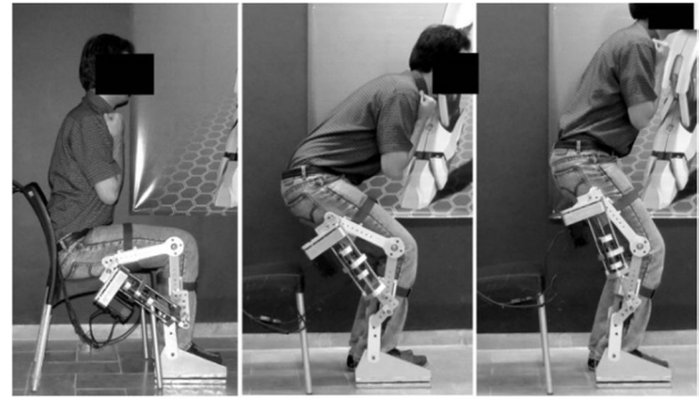
Fig. 12 Snapshots of the sit-to-stand movement with the help of the knee exoskeleton
