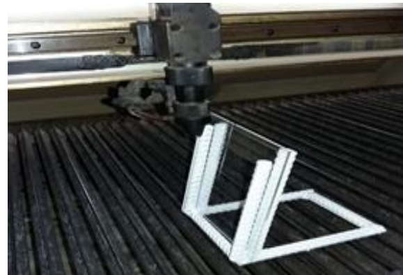
Fig. 3 Experimental determining of the focal plane position of the used CO 2 laser machine
