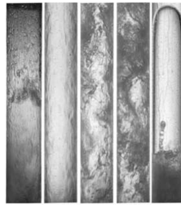
Fig. 6 Flow patterns in tube with inner diameter of 80 mm a) slug, b) churn, c) churn-annular, d) annular, e) reverse flow
