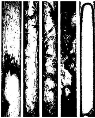
Fig. 4 Binary Images of Flow patterns in tube with inner diameter of 60 mm
