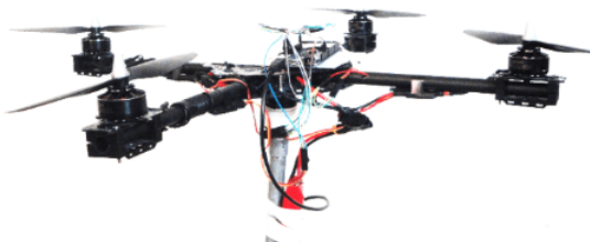
Fig. 10 Quadrotor on the experiment base with three degree of freedom
