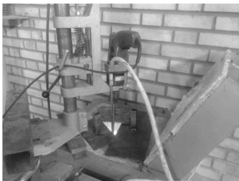
Fig. 2 The stir casting system used in this study
