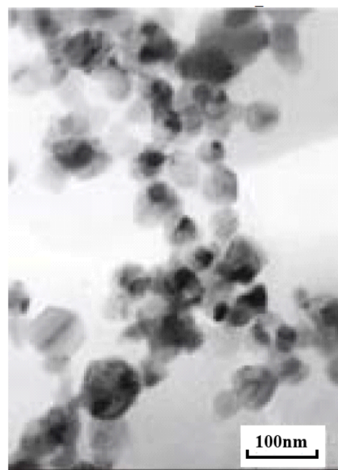
Fig. 1 TEM images of SiC nanoparticles used in this study
