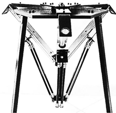
Fig.2 Manufactury model of the 3-[P2(US)] parallel manipulator
