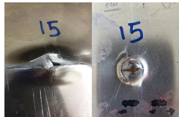
Fig. 17 Target No.15: front side (left) and back side (right) view under the penetration of hemispherical projectile in 55J impact
