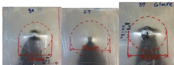
Fig. 13 Damage zone propagation on target No.10 (hemispherical projectile), No.27 (flat projectile) and No.37 (conical 90° projectile)
