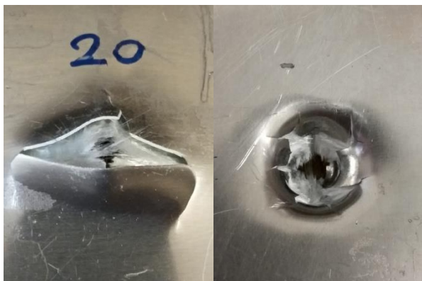
Fig. 23 Target No.20: front side (left) and back side (right) view under the penetration of hemispherical projectile in 70J impact
