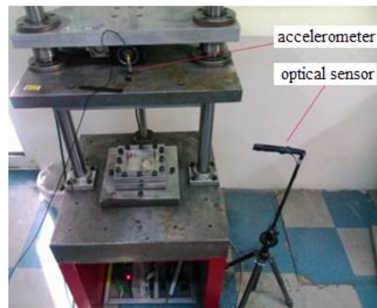
Fig. 6 Drop weight testing machine accelerometer and optical sensor
