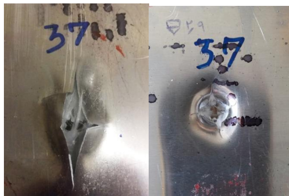
Fig. 12 Target No.37: front side (left) and back side (right) view under the penetration of conical 90° projectile in 40J impact
