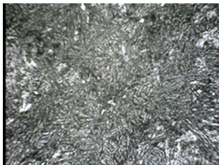
Fig. 5 The micro structure of the bainite phase
