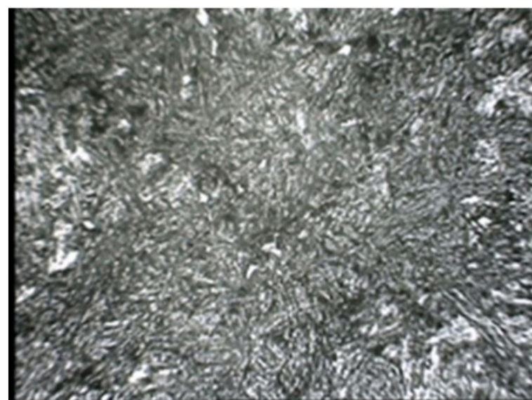
Fig. 5 The micro structure of the bainite phase
