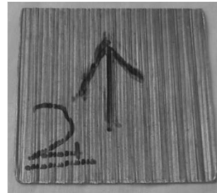
Fig. 6 The Al 5052 sheet fabricated by two passes of CGP
