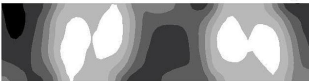
Fig. 8 Effective strain distribution in Al 5052 sheet subjected to one pass of CGP process
