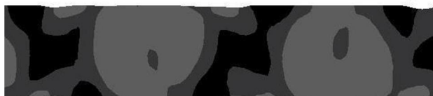
Fig. 9 Effective strain distribution in Al 5052 sheet subjected to two passes of CGP process
