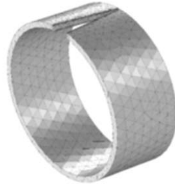
Fig.4 model meshed with tetrahedral element.
