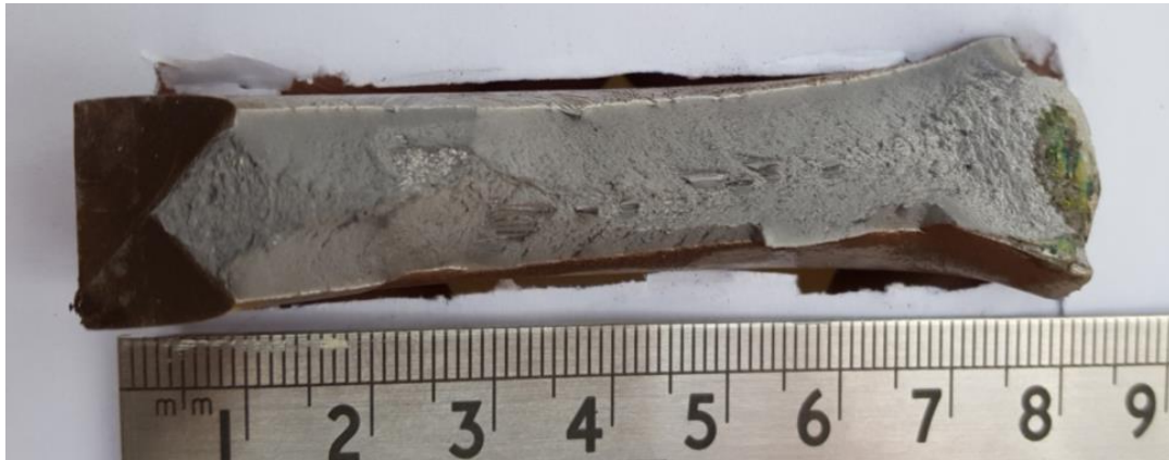
Fig. 15 Fracture surface of right part of DWTT specimen with crack growth direction from left to right
