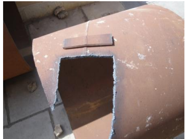
Fig. 3 Specimen machined from an actual gas pipe with spiral seam weld
