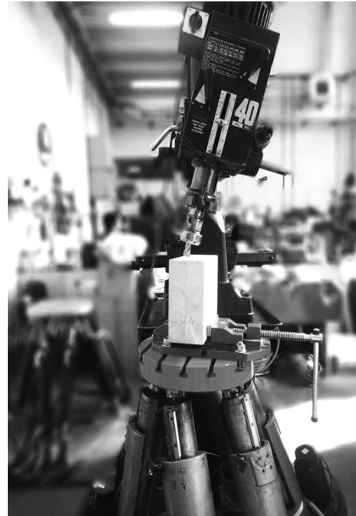
Fig. 2 Rotating the milling machine's head
