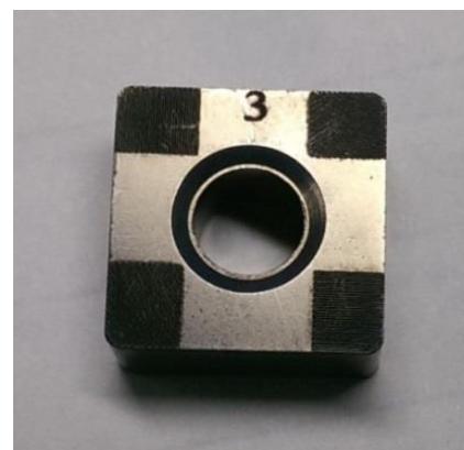
Fig. 4 Cutting insert image after creating the micro-texture
