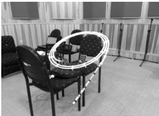
Fig. 4 Practical pulse reflectometer which made for measuring input impedance of ney. The ney under investigation is seen at the end of source tube
