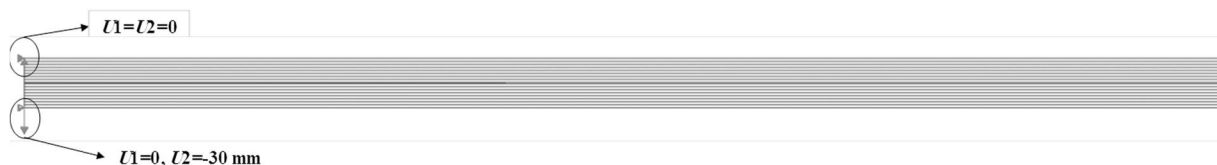
Fig. 6 DCB specimens boundary conditions
