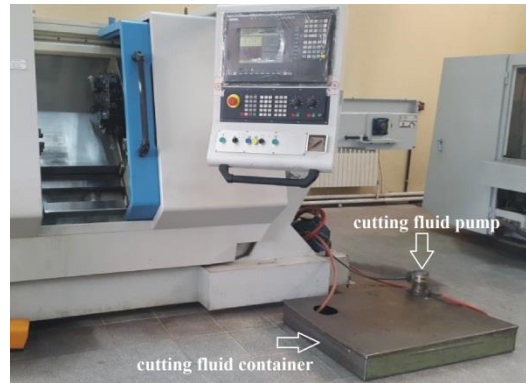
Fig. 1 CNC turning machine and designed cutting fluid container
