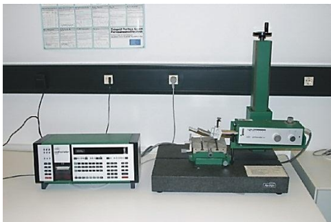
Fig. 2 Surface roughness testing machine
