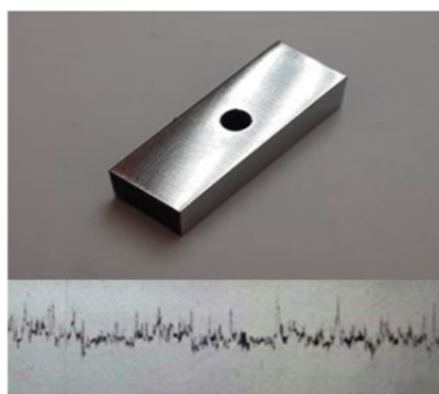
Fig. 20 Workpiece with 55 HRC hardness and its surface profile after RAJM process (mesh: 150 and N=100 rpm)
