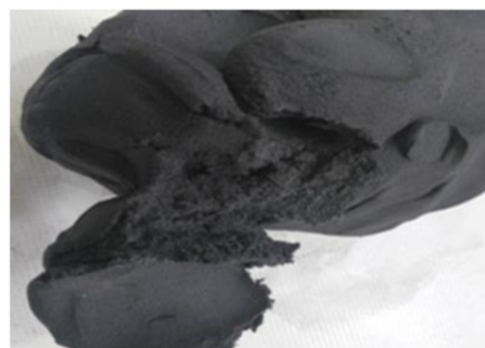
Fig. 6 Abrasive compound with paraffin and grease
