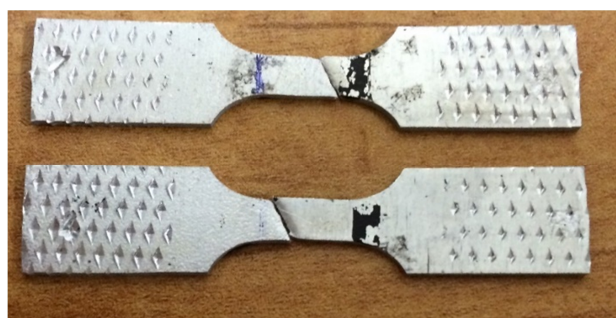
Fig. 2 fracture of sample after uniaxial tensile test
