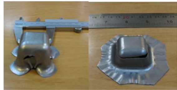
Fig. 15 Comparison of Al(0.4mm)/St(1.6mm) sheet forming with traditional (left) and hydromechanical (right) methods
