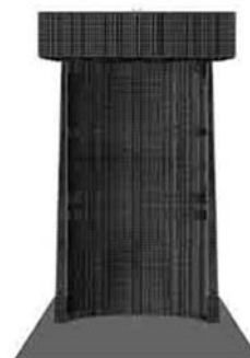
Fig. 5 A view of longitudinal section in the moment that stationary tube is impacted by striking mass in Abaqus
