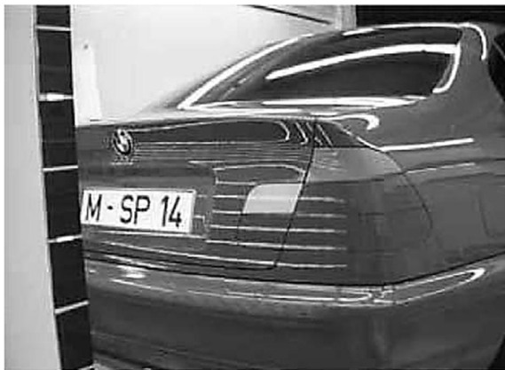
Fig. 2 Application of highlight bands in quality appearance evaluation of a car body [23].
