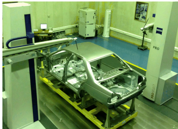
Fig. 18 Surface scanning of a car's roof using CMM
