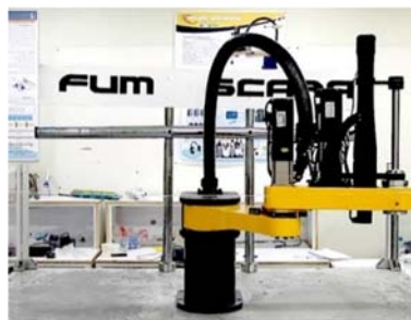
Fig. 11 The FUM SCARA robot designed and built at the Ferdowsi university of Mashhad, FUM Robotics Lab
