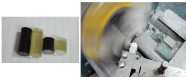
Fig. 4 Specimens that are made by using lathe machine
