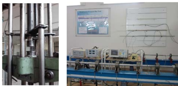
Fig. 5 Split Hopkinson Pressure Bar and Uniaxial Compression Tests
