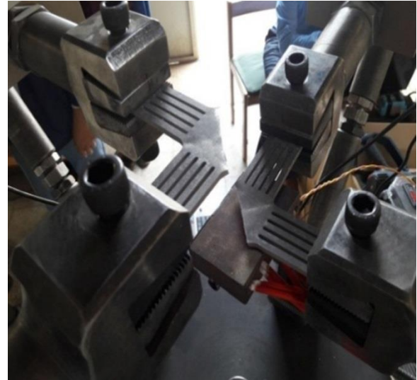
Fig. 8 The cruciform specimen fracture from Al. alloy 5083
