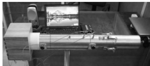
Fig. 2 Impedance tube used in this investigation
