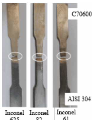
Fig. 19 The image of fracture zone of the fractured specimens in tensile test
