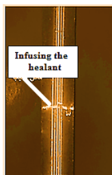
Fig. 2 The damage generated via Charpy impact test and infusing the healing agent.
