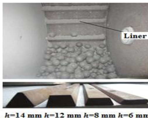
Fig. 4 Liners used and position of lifters in experiment SAG mill
