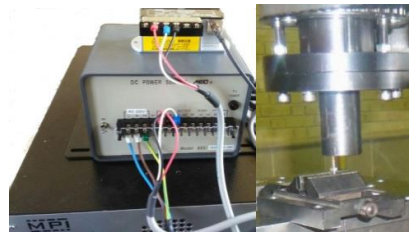
Fig. 8 Measurement of amplitude by gap sensor
