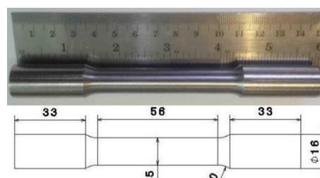
Fig. 13 The specimen used for the tension test
