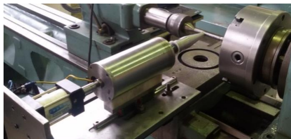
Fig. 10 Assembling of UPT equipment on the lathe
