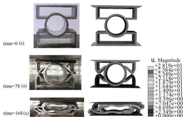
Fig. 14 Comparison of the collapse of an empty specimen under loading angle of 90° by the experimental and numerical methods
