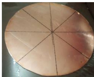
Fig. 5 Circular copper plate before the loading
