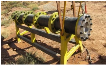
Fig. 3 The real view of the explosive shock tube
