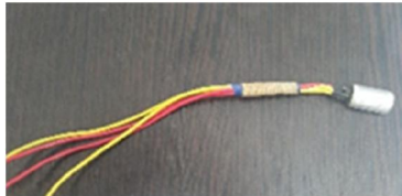
Fig. 4 The utilized capsule and charge for the explosive charge
