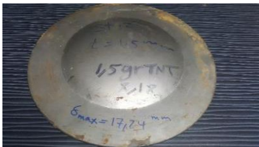
Fig. 8 Deflection of 1.5 mm steel plate during loading 1.5 gram T.N.T
