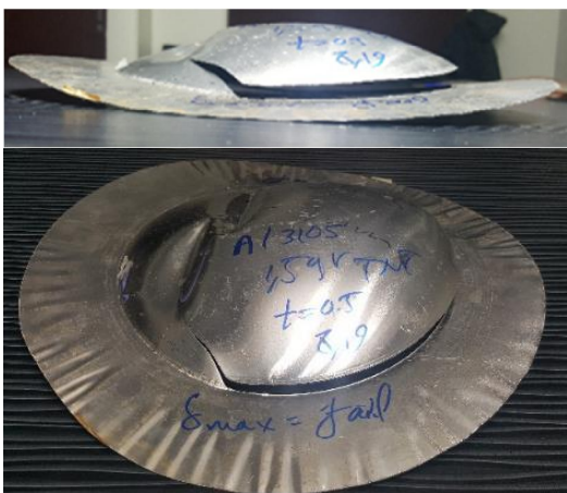
Fig. 6 Ripping 0.5 millimeter aluminum plate during loading 1.5 gram T.N.T
